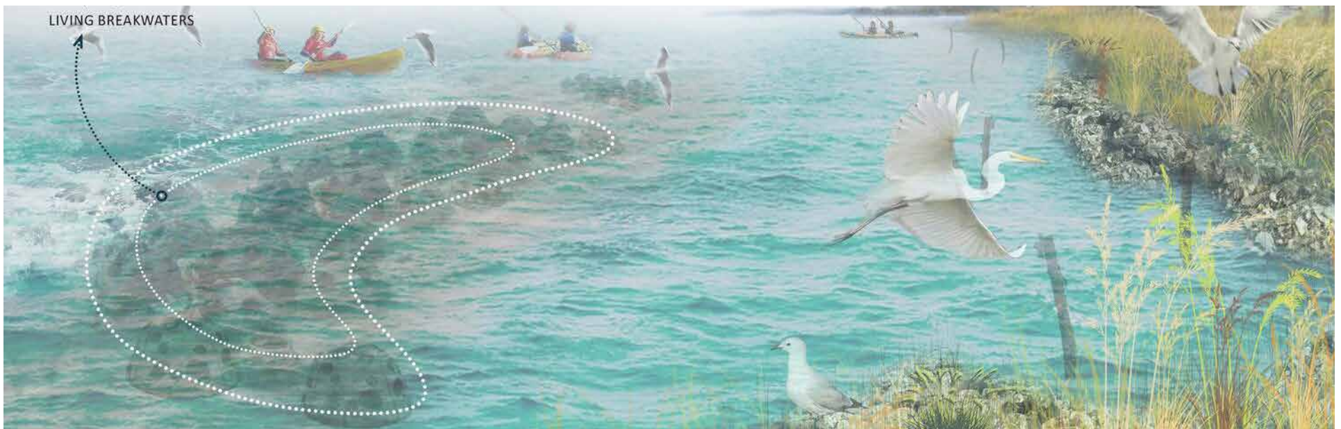
NC State's Coastal Dynamics Design Lab developed renderings of living breakwaters for Nags Head's Estuarine Shoreline. Like the concepts in this plan, these concepts used reef balls rather than oysters, which cannot thrive in Roanoke Sound's low salinity. Credit: NCSU Coastal Dynamics
