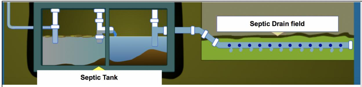
**Figure 3. Septic System Layout.** This is a diagram of a septic tank and drainfield connected to a house, filtering wastewater.
