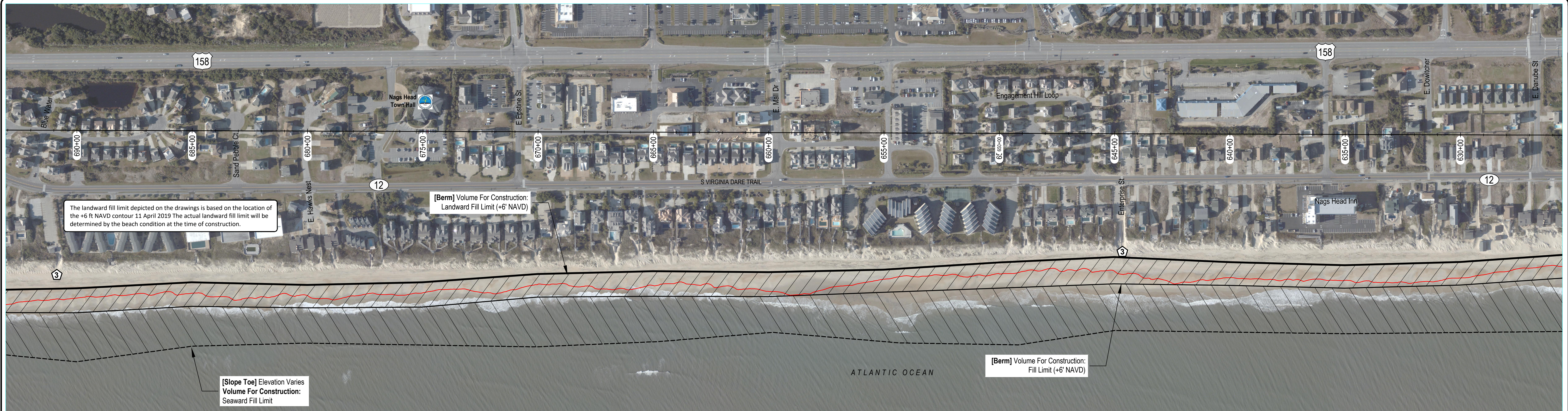
Reach 1 (Sta 497+00 to 790+00) Volume For Construction: 1,758,000 cy
