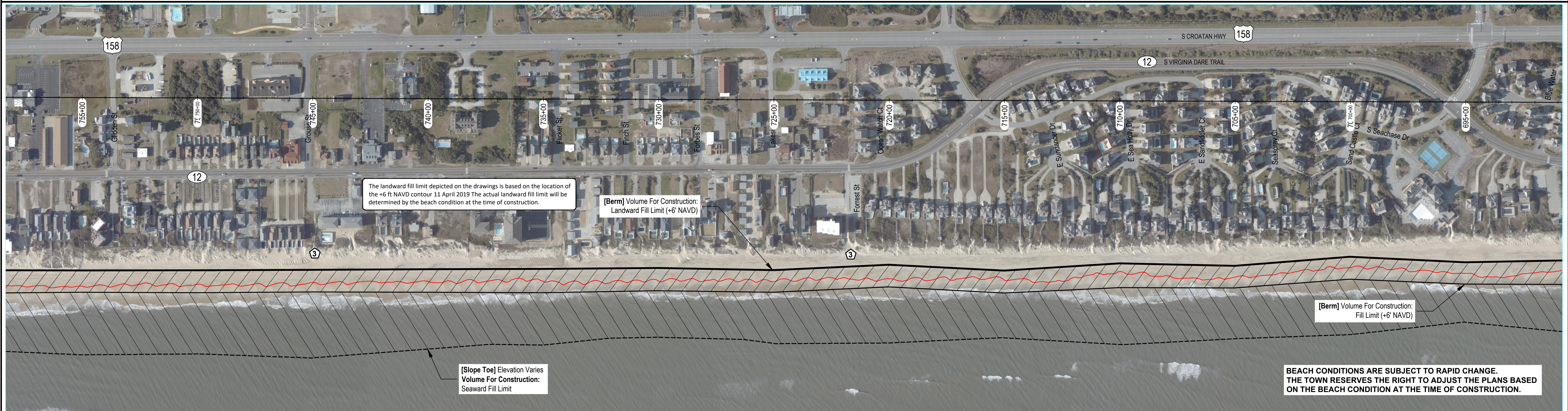
Reach 1 (Sta 497+00 to 790+00) Volume For Construction: 1,758,000 cy
