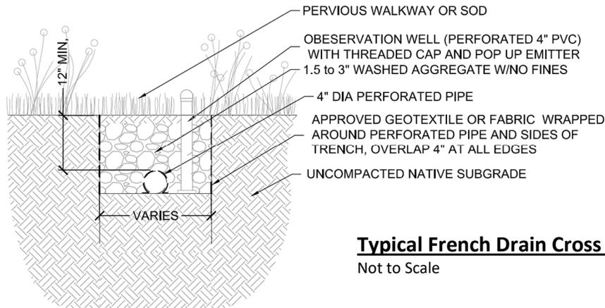
**Typical French Drain Cross Section**
